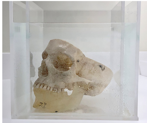
Fig. 1. Dry skull and 3-dimensional (3-D)-printed mandible placed in a Plexiglas box with water-filled compartments simulating soft tissue attenuation during cone beam computed tomography (CBCT).
