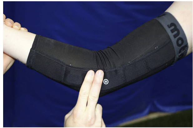
Figure 2 Wearable baseball compression sleeve with sensor device at medial elbow. The sensor is placed inside a medial elbow pocket and outputs accelerometer and gyroscope data to be recorded by a mobile phone application (motusTHROW, version 8.3.3). The wearable device records elbow torque (in newton meters), arm slot (in degrees), arm speed (in rotations per minute), and shoulder rotation (in degrees). The device is placed so that the sensor rests 3.81 cm (1.5 in) distal to the medial epicondyle of the humerus, as directed by the device manufacturer's instructions. The medial epicondyle is depicted by the circle on the sleeve.
