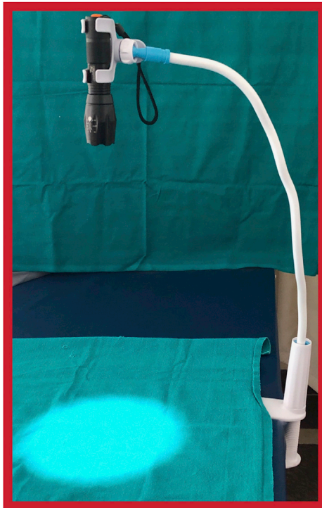
Fig 1. Light-emitting diode torch fixed on mobile phone stand.
