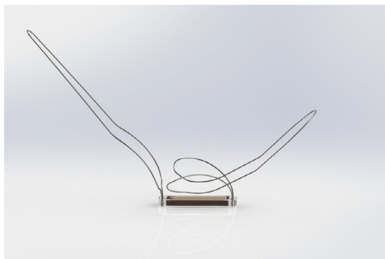
Fig 3. Cordella PA sensor system. Used with permission of Endotronix.
