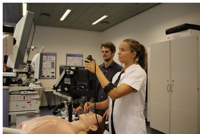
Fig. 2. Experimental setup with the participant performing a full bronchoscopy while wearing the Myo Armband and the first author performing a live rating.
