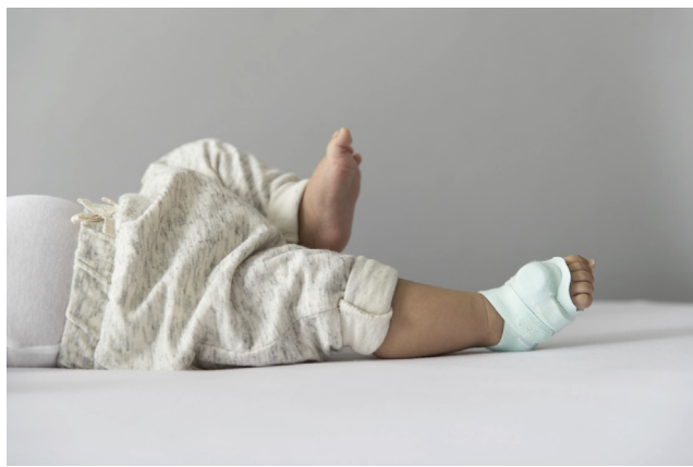
Figure 1. The OSS collects HR, SpO 2 , and surface temperature data from sleeping infants.
