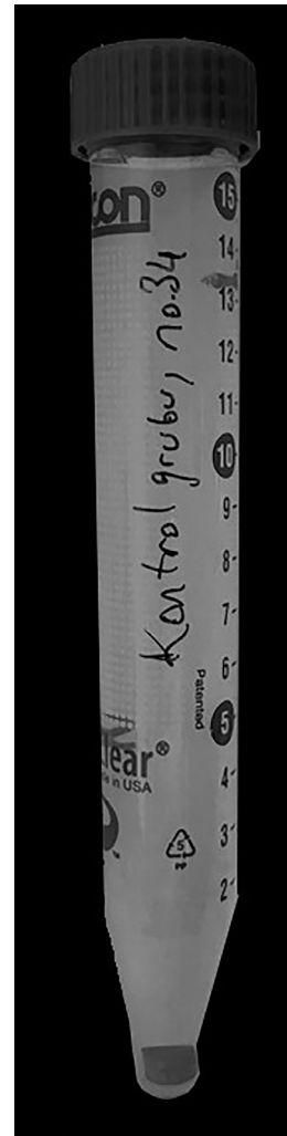
Fig. 1. One of the prepared samples. The cylindrical disk of amalgam is depicted at the bottom of the tube.
