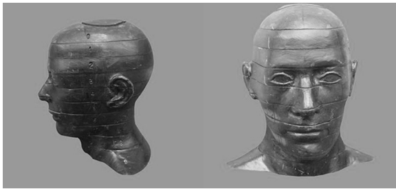
Figure 1. Left lateral (L) and anterior (R) views of the RANDO phantom used in this study. An adult male human skull is embedded in the tissue-equivalent material. The horizontal lines are the levels, numbered on the left, which were separated for placement of the optically stimulated luminescence (OSL) dosimeters in the appropriate tissue locations.
