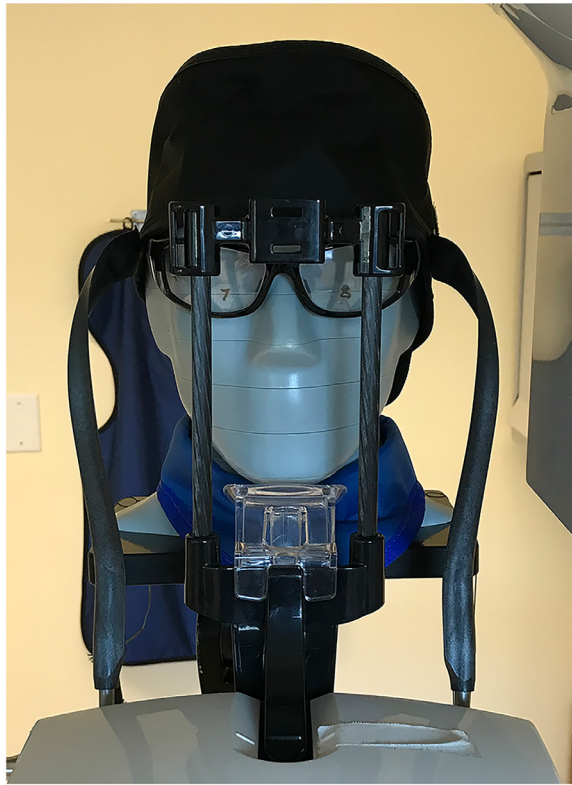
Fig. 2. Full shielding applied to the adult male anthropomorphic phantom during the limited field of view cone beam computed tomography scans.
