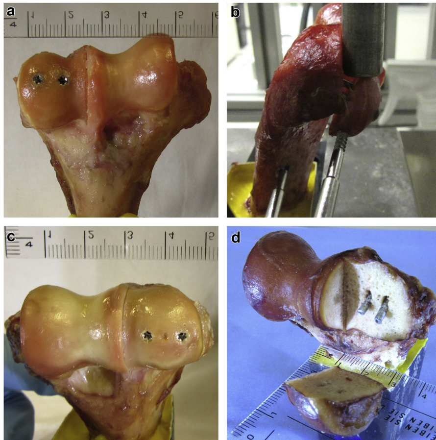
Figure 3 Constructs and failure mode. (a) Titanium screw construct with 2 headless screws buried under the cartilage surface. (b) Distal screw cutout—the most observed failure mode in this study—in a titanium screw construct. (c) Magnesium screw construct. (d) Screw breakage, which occurred in 2 magnesium screw constructs after 71,099 and 60,536 cycles.
