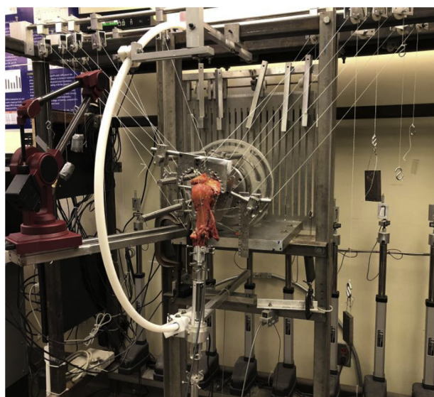
Figure 1 Anterolateral view of custom shoulder-testing system with right shoulder mounted in 0° of glenohumeral abduction.
