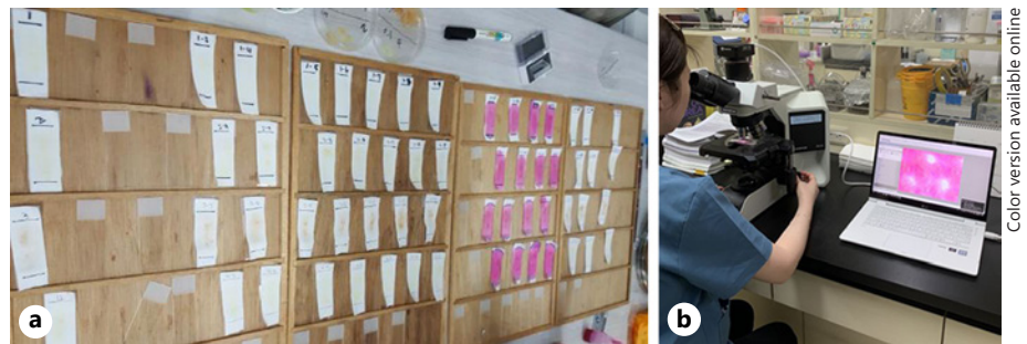
Fig. 2. a Fabric was stained using Calberla's fuchsin solution. b Counting number of pollen using a microscope.
