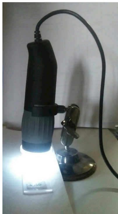
Fig 2. Stable perpendicular placement of a high-magnification universal serial bus dermatoscope (Escopie USB videodermatoscope; Timpac Healthcare Pvt Ltd, New Delhi, India) rimming a potassium hydroxide mount of extracted hair follicles placed over a glass slide.
