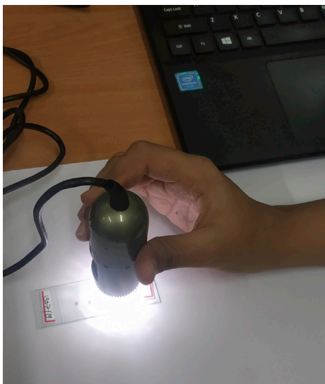
Fig 1. Video dermoscope placed over a stained slide on a white background under polarized mode.
