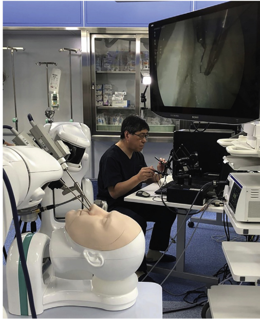
Fig. 2. Setup of a novel robot designed for pure transnasal skull base work. (From Marinho MM, Harada K, Morita A, et al. SmartArm: Integration and validation of a versatile surgical robotic system for constrained workspaces. Int J Med Robotics Comput Assist Surg. January 2020:e2053; with permission.)
