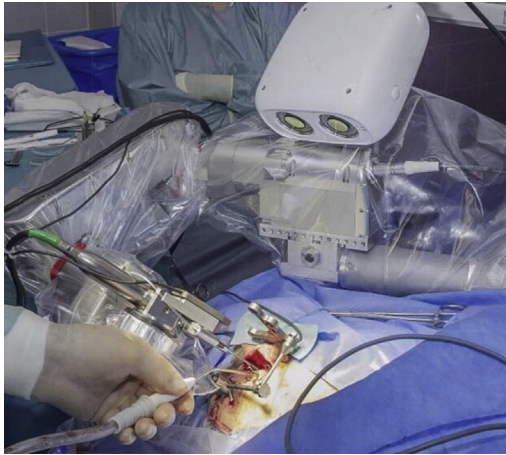
Fig. 4. HEARO system showing the IGS system ( white box houses infrared tracking cameras) monitoring the robotic arm relative to the patient. The human hand is holding suction-irrigation clearing away debris so that humans can visualize the interaction between the end effector and the patient. (From PLoS One. 2019; 14(8): e0220543. Published online 2019 Aug 2. https://doi.org/10.1371/journal.pone.0220543 .)
