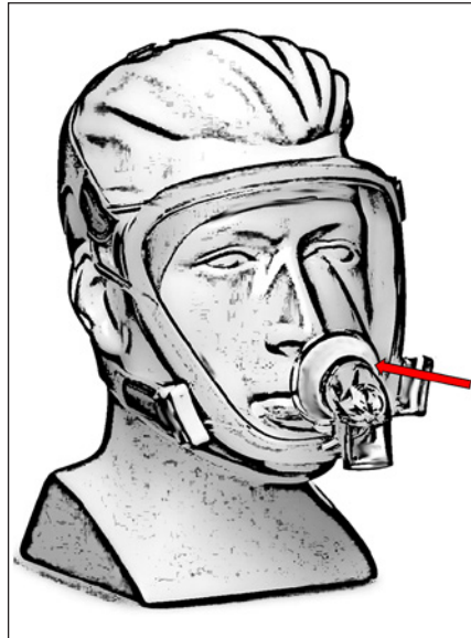
Fig. 11. Vented total-face mask. The arrow indicates the intentional leak port.
