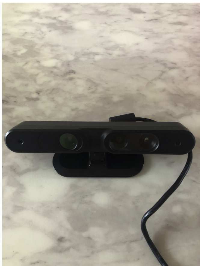
Fig. 1. The camera set of the PrimeSense 3D system.
