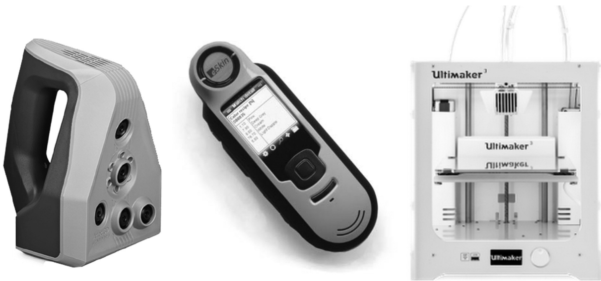
FIGURE 1. Instruments for noncontact facial topography mapping and 3D printing of orbital prosthesis. Left: Full Color 3D scanner. Center: Colorimeter. Right: 3D printer.
